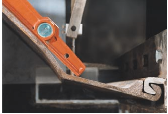
Figure 5b: Concentration of the plastic deformations in the corner of the section angle.
